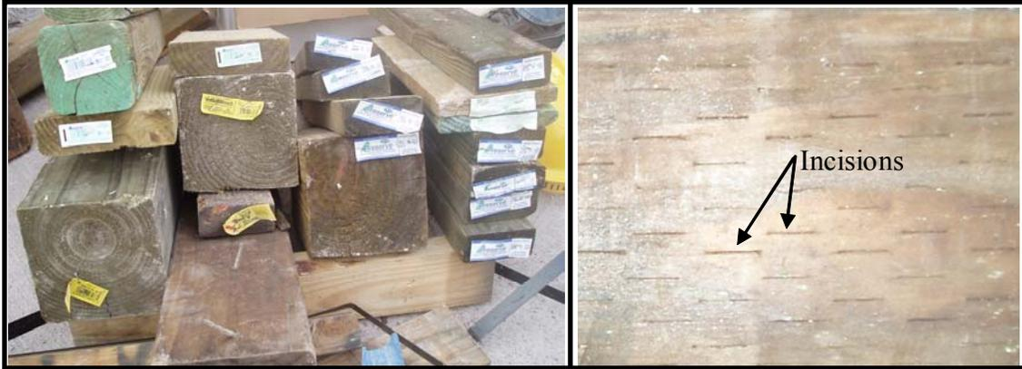
Figure 1: Treated Wood “Identifiers” in C&D wood waste. End tags show the type of chemical contained in treated wood (left). Wood that contains incisions (right) is also treated.
