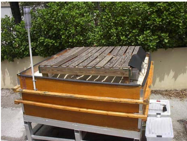
Figure 1: Deck used to evaluate leachable arsenic and chromium
