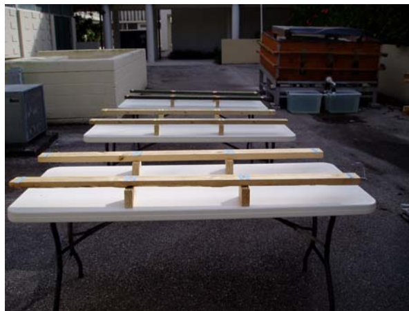
Figure 2: Outdoor wipe stations to evaluate dislodgeable arsenic and chromium
