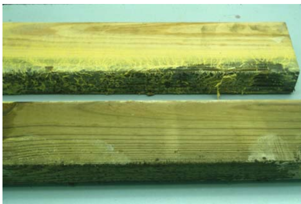
Figure 3. Meruliporia incrassata (TFFH 294) decay of CCA-treated wood. Top lumber is nontreated southern yellow pine and bottom is CCA-treated.
